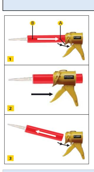
◆ Pull and hold the clutch (A). Insert the cartridge (B). Release clutch.
